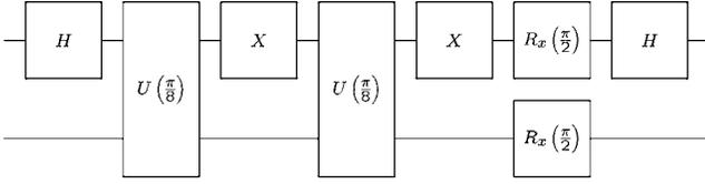
FIG. 8. Circuit diagram for the CNOT gate.
