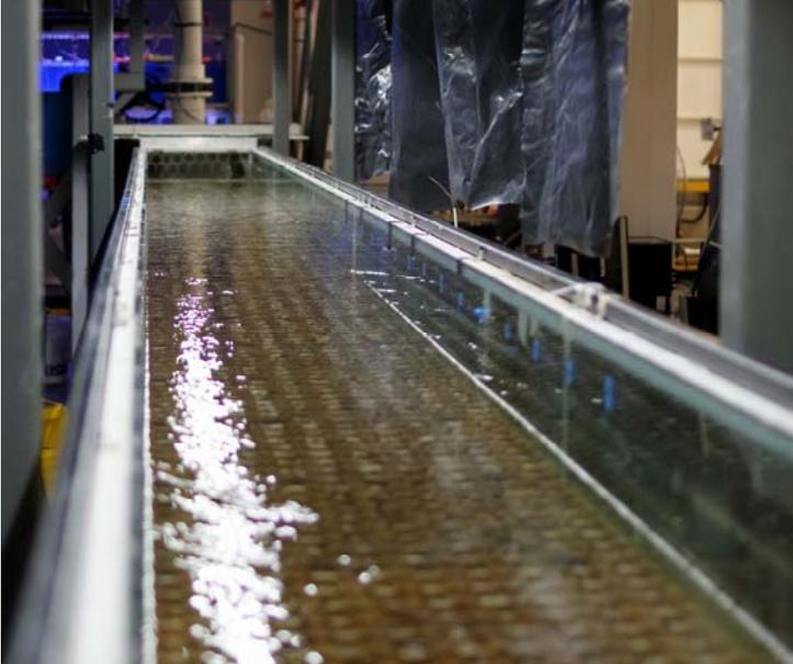
(B) Recirculation water tunnel:  $B = 0.25$  m,  $\theta = 0$ ,  $V \sim 0.05$  m/s,  $d = 0.26$  m, flow motion from left to right
