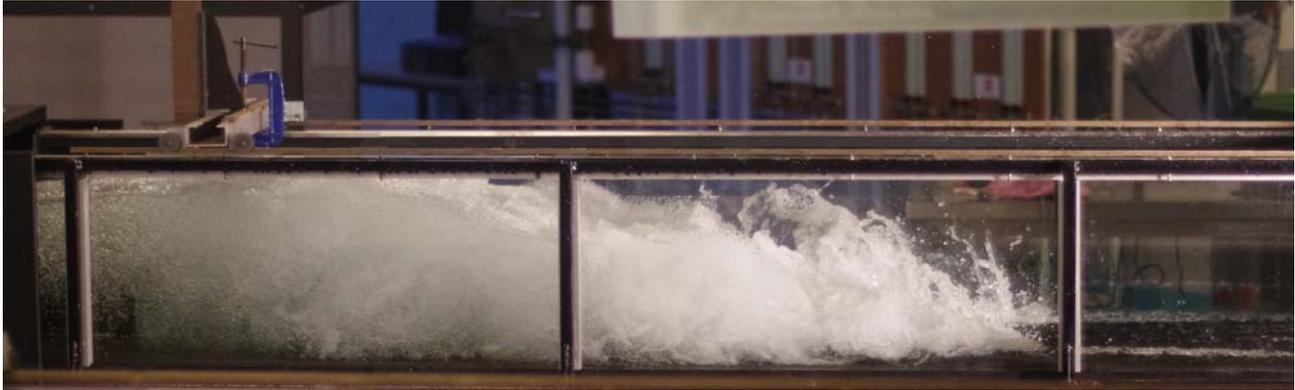
Fig. 3 - Air bubble entrainment in a hydraulic jump with a marked roller
