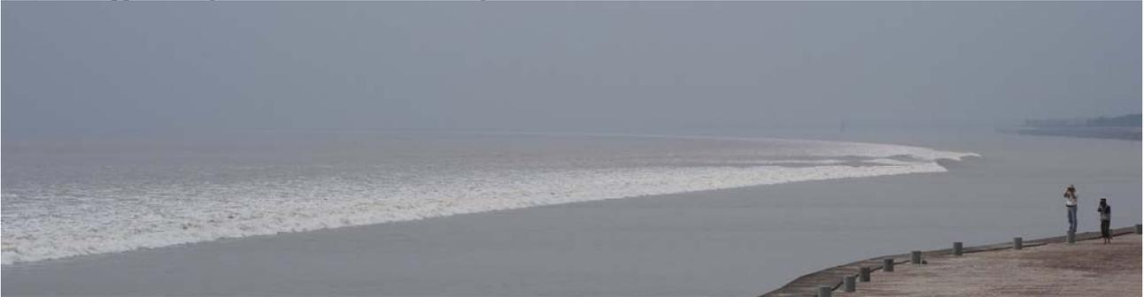
(B2) Bore roller propagating (from left to right) parallel to the seawall at Qilimiao at 13:20 - The roller height was about 2.5 m to 3 m, the bore celerity 4 m/s to 5 m/s and  $Fr \sim 2$  - Shutter speed: 1/6,400 s
