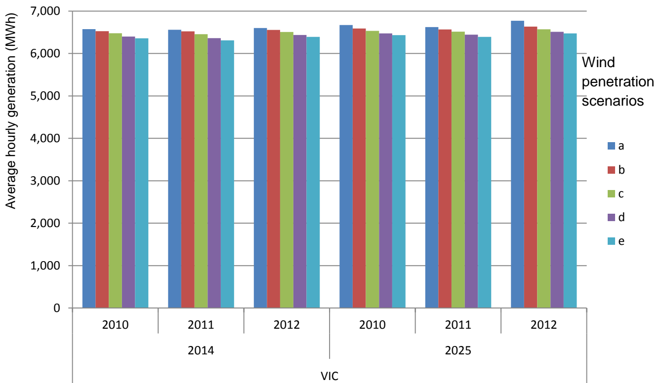
Figure 9: Comparing wind power, weather and growth effects on the VIC's average hourly generator energy
