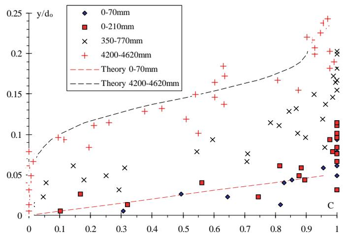
Figure 8 Dimensionless void fraction distributions behind the wave front leading edge ( $Q(t = 0+) = 0.070 \text{ m}^3 \text{ s}$ ,  $h = 0.07 \text{ m}$ ,  $W = 0.5 \text{ m}$ , Step 16,  $C_s = 2.86 \text{ ms}^{-1}$ ,  $X' = 0.3 \text{ m}$ )—Comparison with Eqs (5) and (6).
