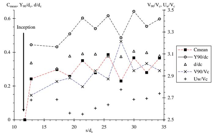
Figure 4 Longitudinal distributions of mean air contents  $C_{mean}$ , dimensionless air–water depth  $Y_{90}/d_c$ , clearwater depth  $d/d_c$ , air–water velocity  $V_{90}/V_c$  and mean flow velocity  $U_w/V_c$ —Stepped chute:  $16^\circ$  slope,  $h = 0.05$  m,  $d_c/h = 1.7$  (Yasuda and Chanson, 2003).
