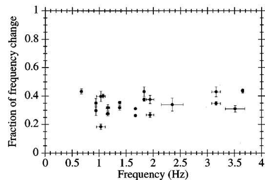
FIG. 5. Plot of fractional change in rotation frequency vs rotation frequency for CuO particles. The change in rotation frequency is due to rotation of a  $\lambda/4$  plate by  $45^\circ$ , changing the polarization of the beam from plane polarized to circularly polarized. The error bars reflect the uncertainties in frequency measurements on the individual particles.
