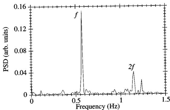
FIG. 3. Spectrum obtained from a CuO particle with two protrusions resulting in strong peaks at both  $f$  and  $2f$ , where  $f$  is the actual rotation frequency of the particle. That  $f$  is indeed the true rotation frequency of the particle was verified by observation of a video recording made simultaneously with the taking of the data shown in Fig. 2.
