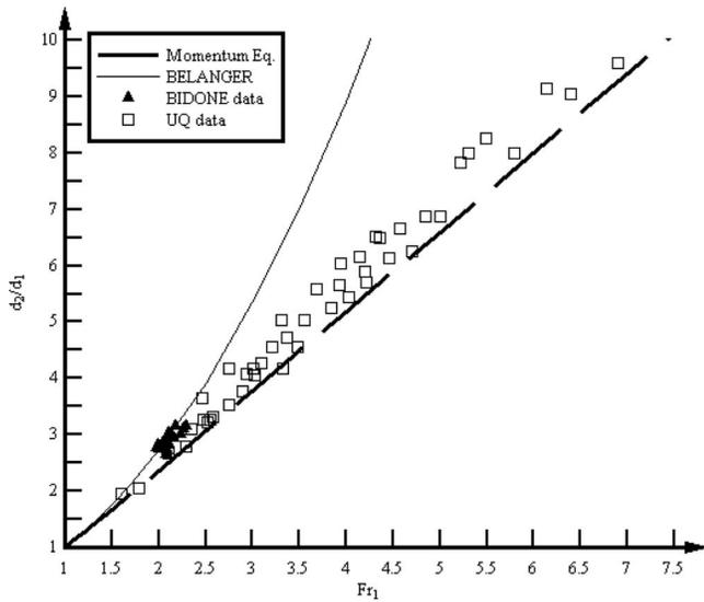
**Fig. 2.** Ratio of conjugate depths for a hydraulic jump in a rectangular, horizontal, and prismatic channel: comparison of Eq. (1), Eq. (3) by Bélanger (1828), experimental data by Bidone (1819), and experiments in a 0.5-m-wide channel at the University of Queensland
