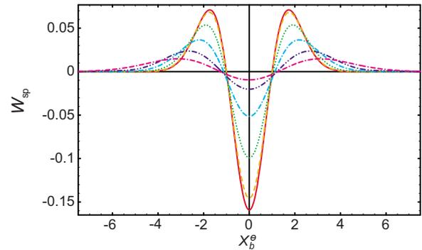
FIG. 4. (Color online) Cuts through the center of the Wigner functions  $W_{\text{SP}}(X_b^\theta)$  for varying value of squeezing. (solid) single photon using the moment definition given by Eq. (18), (dash)  $V_s=-1$  dB, (dot)  $V_s=-3$  dB, (dash-dot)  $V_s=-5$  dB, (dash-dot-dot)  $V_s=-7$  dB, and (dash-dash-dot)  $V_s=-9$  dB.
