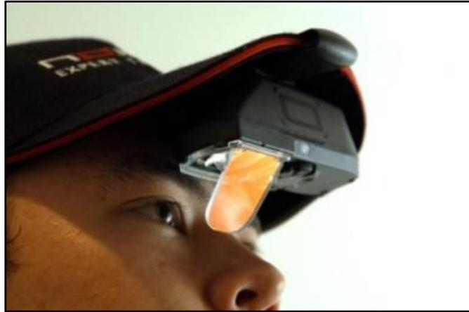
Figure 1. Transparent Monocular Head-Mounted Display
