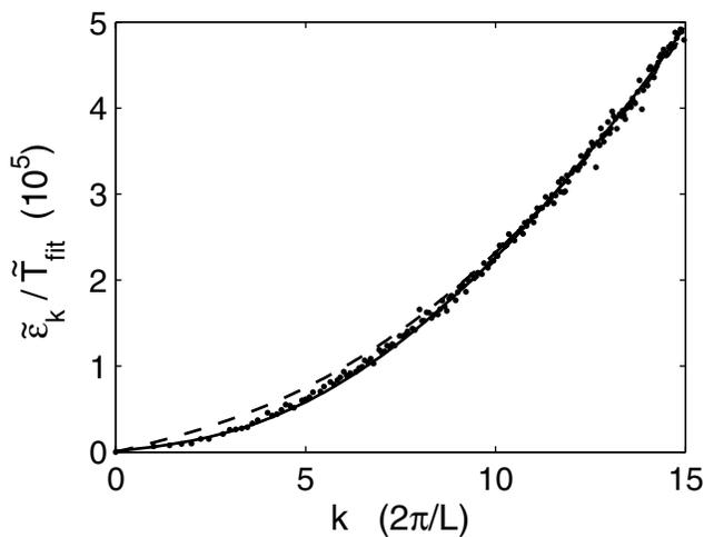
FIG. 4. Comparison of dispersion relations for  $\tilde{E} = 4000$  with  $\langle N_0 \rangle / N = 0.279$ . The dots are a plot of the RHS of Eq. (8) and the lines plot  $\tilde{\epsilon}_k / \tilde{T}_{\text{fit}}$ . The dashed line is for the Bogoliubov dispersion relation with  $\tilde{T}_{\text{fit}} = 0.193$ , and the solid line is for the second order theory of Ref. [3] with  $\tilde{T}_{\text{fit}} = 0.201$ .
