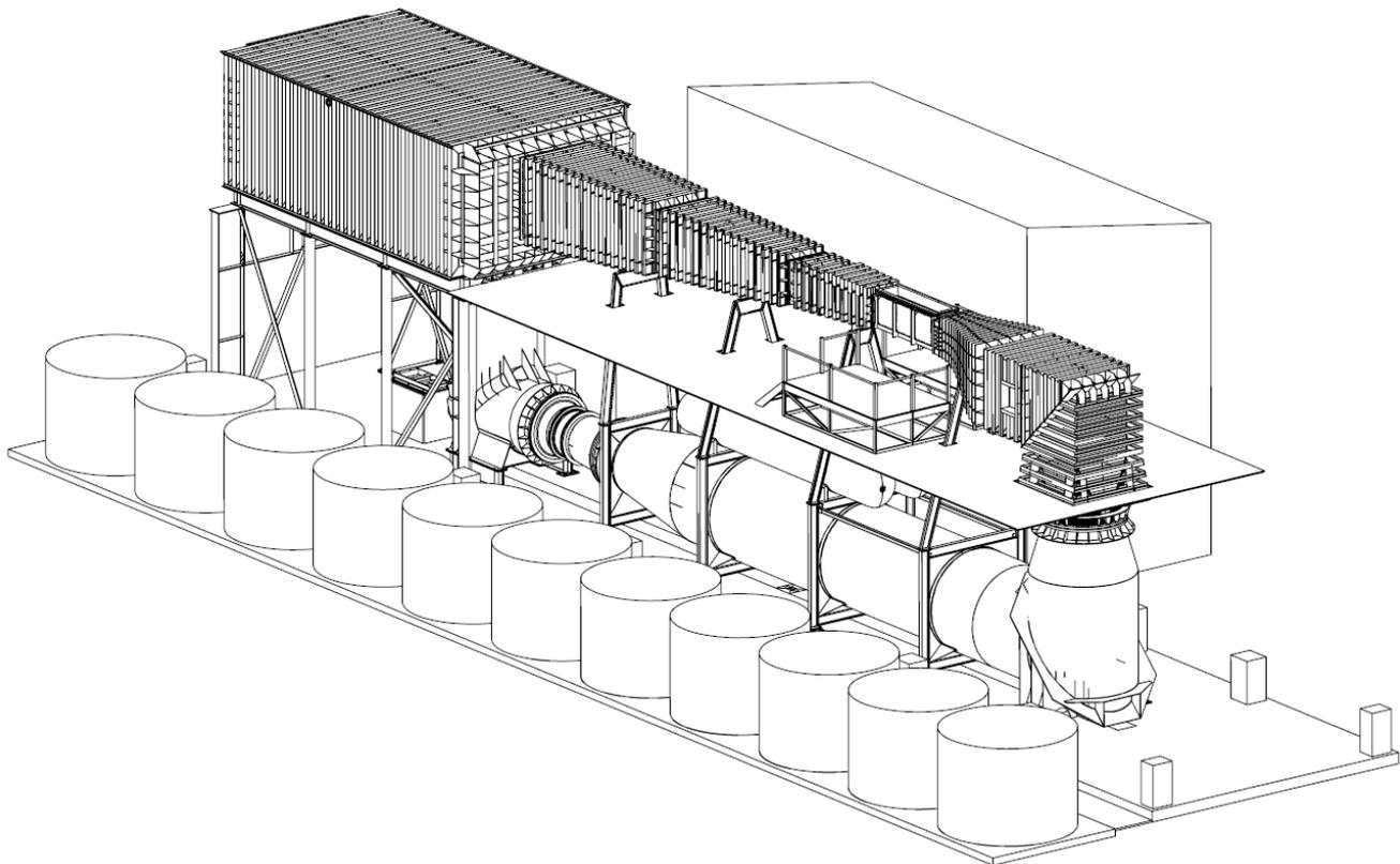
Figure 1. Cavitation tunnel general arrangement – 3 dimensional view
