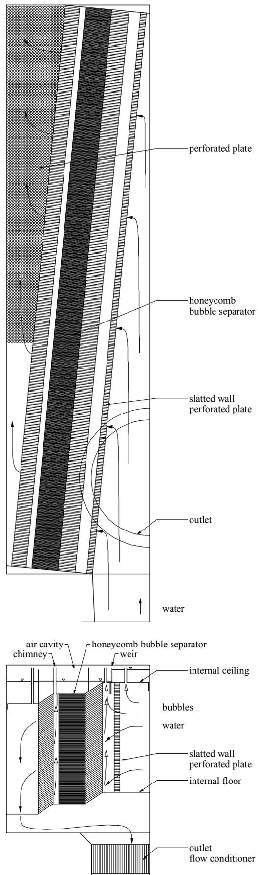
Figure 2 Horizontal and vertical half sections of the downstream tank
