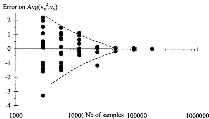
**Fig. 1.** Effects of data sample size on turbulence characteristics in a 0.5-m-wide, 12-m-long open channel [flow conditions:  $Q=0.0404 \text{ m}^3/\text{s}$ ,  $W=0.5 \text{ m}$ ,  $d=0.096 \text{ m}$ ,  $z=27.2 \text{ mm}$ , micro ADV (16 MHz) with 2D sidelooking head, sampling rate=50 Hz; velocity range=1 m/s]
