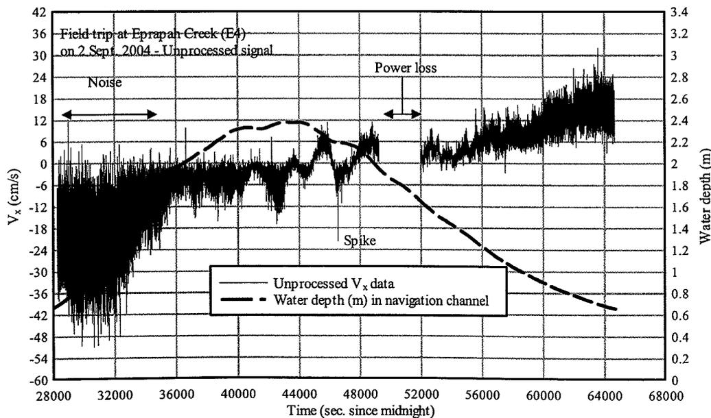
**Fig. 3.** Field data from ADV deployment in a small estuary: streamwise velocity  $V_x$  component (positive downstream, unprocessed “raw” signal) and measured water depth [time in seconds since midnight field work: Sept. 2, 2004, ADV (10 MHz) with 3D downlooking head; sampling rate=25 Hz, continuous sampling; velocity range=0.30 m/s; sampling volume located 0.052 m above bed and 10.8 m from left bank]
