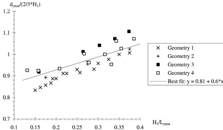
Fig. 2. Dimensionless water depth on the weir crest (measured at  $x/L_{crest} = 0.46$ ).
