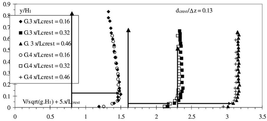
(A) Dimensionless velocity distributions  $V/\sqrt{g^*H_1}$  as functions of  $y/H_1$  - The horizontal axis is  $V/\sqrt{g^*H_1} + 5*x/L_{crest}$ .
