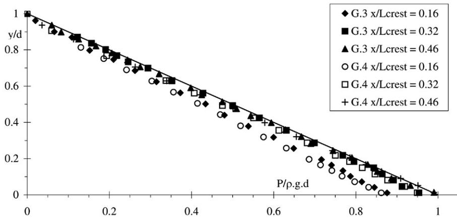
(B) Dimensionless pressure distributions  $P/(\rho^*g*d)$  as function of  $y/d$  - Comparison with the hydrostatic pressure distribution.
