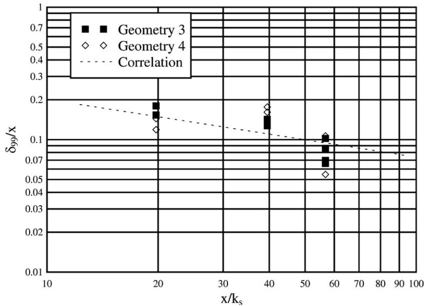
Fig. 5. Dimensionless boundary layer thickness for Geometries 3 and 4 ( $x/L_{\text{crest}} \leq 0.5$ ). Comparison with Eq. (3).
