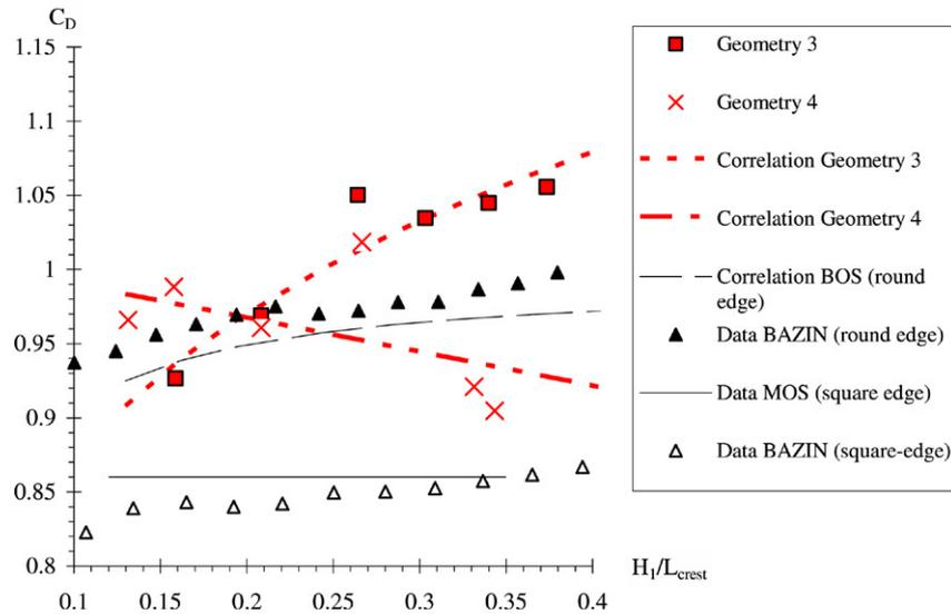
Fig. 6. Dimensionless discharge coefficients for Geometries 3 and 4. Comparison with Eqs. (5) and (6), and previous studies with square-edge [2,13] and rounded edge [2,4].
