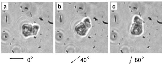
FIG. 1: Three sequential photographs (frames) of a trapped calcite crystal, showing alignment with the plane of polarization of the trapping beam. A  $\lambda/2$  waveplate was rotated by  $20^\circ$  between successive photographs, rotating the plane of polarization by  $40^\circ$ , as shown by the arrows, and exerting an alignment torque on the crystal, causing it to rotate to a new position. This can be used to rotate the particle at a controlled speed, or to control its orientation.
